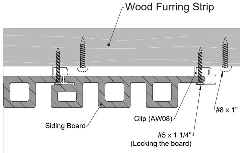
When installing vertically, it is required to lock the Clip (AW08) at the top of the board to allow the remaining board to expand and contract freely.
