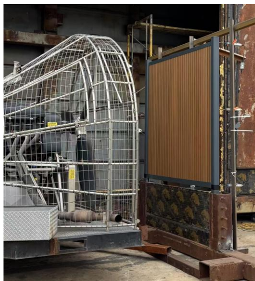
Photo No.2 The specimen under wind load testing
