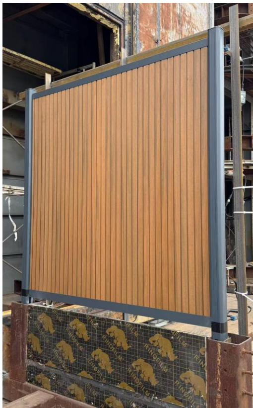
Photo No.1 The specimen before wind load testing
