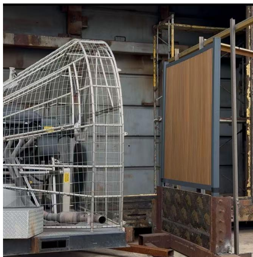
Photo No.3 The specimen after wind load testing
